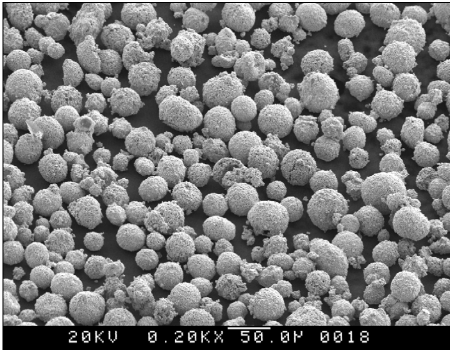
Figure 1: Typical Powder Morphology (SEM 200X)
