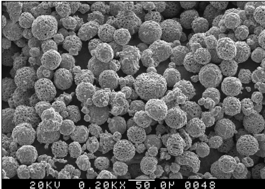
Figure 1: Typical Powder Morphology (SEM 200X)
